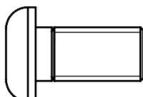
A9.M10X20 TAPER SCREW(FULL THREAD)...4PCS (Pre-installed 2PCS)
