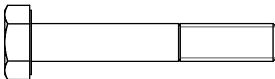
A11.M10X75L HEX HEAD SCREW...3PCS(Pre-installed 1PCS)
